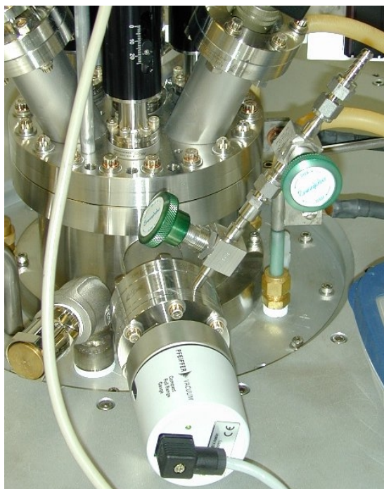
Figure A-7: The pressure gauge and the valves for flowing gas into/through the vacuum space.
