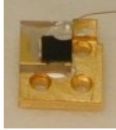
Figure A-1: The sample can be attached to the sample holder using silver paint.
