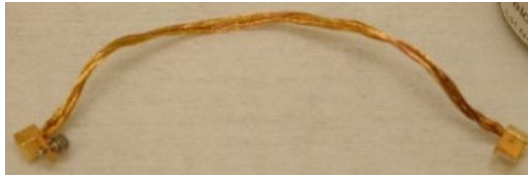
Figure A-2: Copper braid is used for heat sinking the sample and the cantilever.
